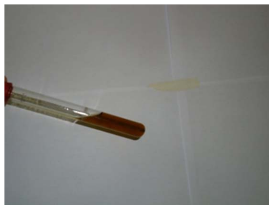
Figure 3. Sample of PAM/PEI, (9/0.3) wt % aged for 49 days at 150°C (302F). [Color figure can be viewed in the online issue, which is available at wileyonlinelibrary.com .]
