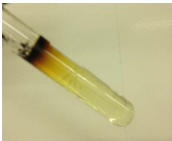
Figure 8. Sample from Berea sandstone core effluents [(PAM/PEI) 9/1 wt % with 6,000 mg/L \text{NH}_4\text{Cl} ] aged beside the core-holder for 5 days. [Color figure can be viewed in the online issue, which is available at wileyonlinelibrary.com.]
